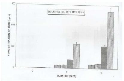
Figure 33. Changes in BOD of "Ngolo" habitat (water) subjected to different simulated crude oil polluted microcosms
